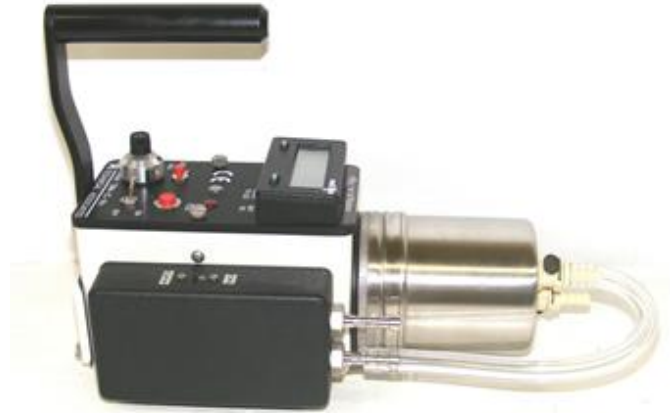
TBM-IC-RN SOLID WALL CHAMBER WITH AIR PUMP
