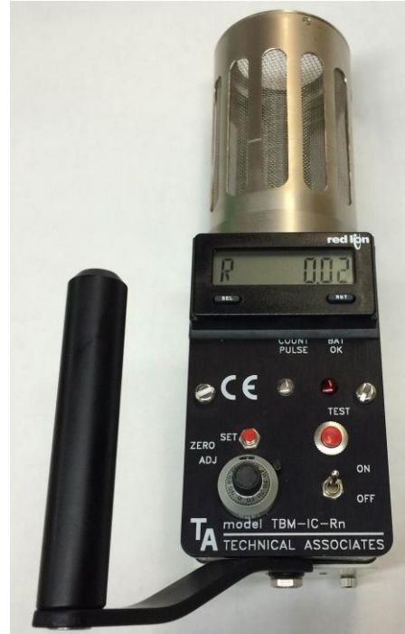
TBM-IC-RN OPEN SCREEN CHAMBER
