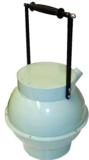
FM-7 Ratemeter (top), BF 3 REM Probe (bottom)
