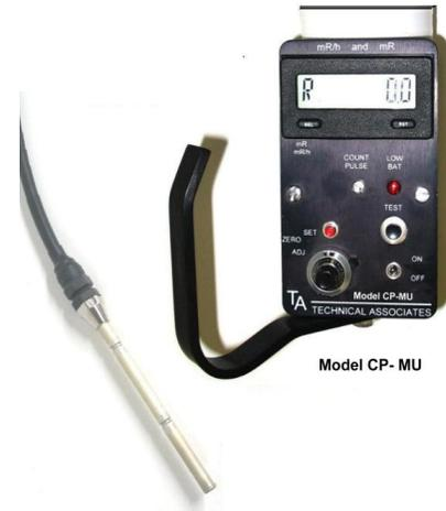
•**APPLICATION:** Because of the extremely high range capability of this instrument and the waterproof construction of the ion chamber detection system, underwater monitoring (and in hot cell monitoring) of Reactor Spent Fuel Elements, Reactor components and dose rate measurements of irradiated objects can now be made easily and at the ranges called for at moderate cost.
